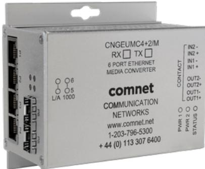
The ComNet CNGEUMC4+2(TX,RX)/M unidirectional media converter with Link Guardian limits network traffic to one way communication between source and destination networks preventing cybersecurity attacks from a non-secured entry point in the network from reaching a secured part of the network. The CNGEUMC4+2(TX,RX)/M provides four 10/100/1000Base-T(X) copper ports and two 1000base-FX SFP ports.
